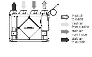
Clearance of 17" (432 mm) in front of the unit is recommended for removal of core. All units feature three foot plug-in power cord with 3-prong plug.
