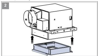
5 Using (4) screws provided with radiation damper assembly, attach radiation damper to the radiation damper casing.
