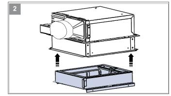
**5** Using (4) screws provided with radiation damper assembly, attach radiation damper to the radiation damper casing.
