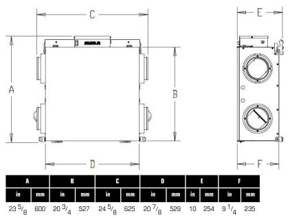
Clearance of 8.5 in. (216mm) in front of the appliance is recommended for removal of core. All appliances feature three foot plug-in power cord with 3-prong plug.
