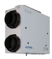
Fantech's ATMO 200E is an Energy Recovery Ventilator designed for higher static pressure applications. The unit brings a continuous supply of fresh air into a home while exhausting an equal amount of contaminated air. The energy recovery core at the center of the unit transfers heat and moisture from incoming air to the outgoing air that was cooled and dried by the building's air conditioner.
