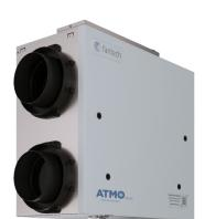
Fantech's, ATMO 150E is an Energy Recovery Ventilator designed for higher static pressure applications. The unit brings a continuous supply of fresh air into a home while exhausting an equal amount of contaminated air. The energy recovery core at the center of the unit transfers heat and moisture from incoming air to the outgoing air that was cooled and dried by the building's air conditioner.
