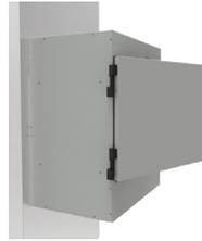
An access door is provided at the front of the unit to permit access to the filters and speed selection switch. Opening the latch on the right side of the unit will permit the door to swing open. A safety door interlock switch cuts the power to the motors for your safety. If needed the door can be removed from the cabinet hinges by holding the top part of the door with one hand and gently tapping on the bottom edge of the door with the other hand to release the door from its hinges.
