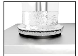
In the case of solid ducting, slide duct over duct connection, screw in place and seal.
