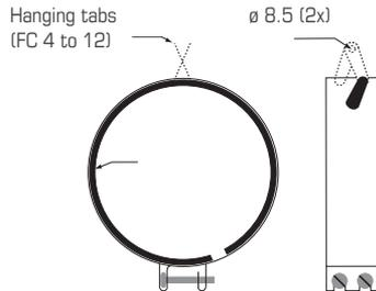
1. Fold out the tabs as shown using needle-nose pliers.
