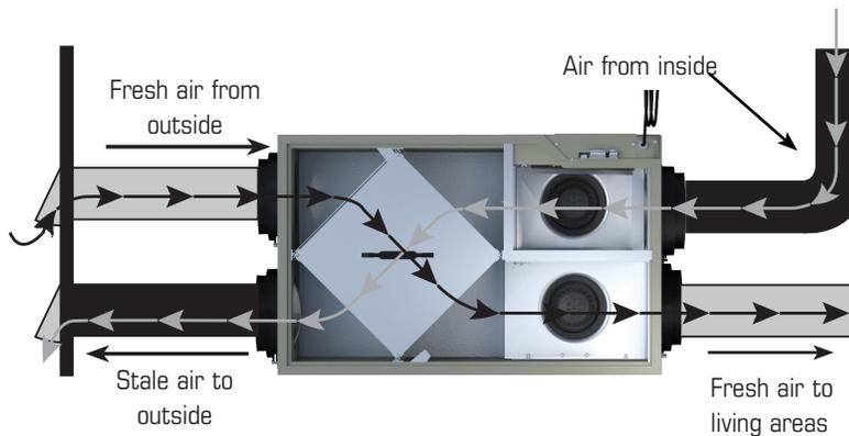
\* Unit air flow should be balanced while ERV is on "Normal" speed and furnace blower is running.
