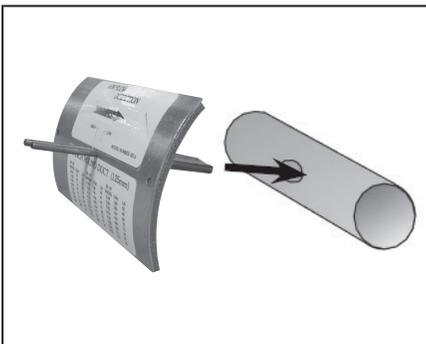
**1** Cut hole in duct and insert flow measuring station. Make sure that the flow measuring station's air direction arrow points in the direction of the airflow. Secure the flow measuring station with aluminum foil tape.
