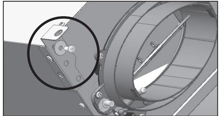
**4** Install bracket and replace screw and washer. Repeat step 3 and 4 on the other side of the unit.
