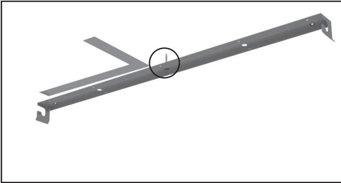
**1** Insert the middle screw with washer in the mounting bracket through the rubber insulator. Ensure the bracket is straight.
