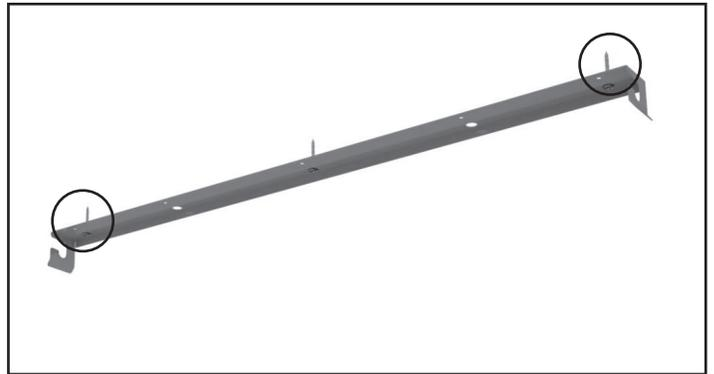
**2** Insert screws with washers on both side of the bracket to secure.
