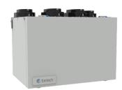
Fantech's, VER 150 is an Energy Recovery Ventilator designed for higher static pressure applications. The unit brings a continuous supply of fresh air into a home while exhausting an equal amount of contaminated air. The energy recovery core at the center of the unit transfers heat and moisture from incoming air to the outgoing air that was cooled and dried by the building's air conditioner.
