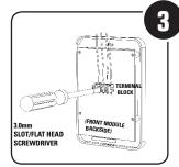
Insert signal wires (4) into the terminal block, located on the backside of the front module.
