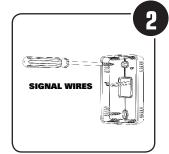
Guide the signal wires (4) through the central opening of the back plate and mount this plate to either a standard electrical device box or directly to the wall using screws. If required, use wall anchors.
