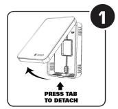
Detach front module from back plate by pressing the tab (located at the top and bottom of the control casing).
