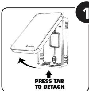
Detach front module from back plate by pressing the tab (located at the top and bottom of the control casing).
