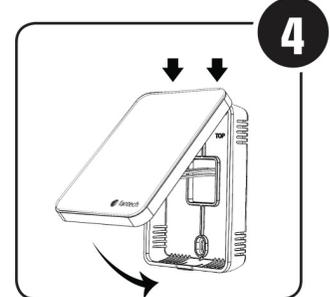
Attach front module to mounted back plate, first by hooking the top of the front module to the top clips of the back plate, then by pressing the bottom of the front module until you hear a 'click'. Ensure the ventilation system operates correctly.
