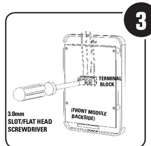
Insert signal wires (4) into the terminal block, located on the backside of the front module. Secure them in place by tightening the terminal screws using a small 3.0 mm slot/flat head screwdriver (not included).
