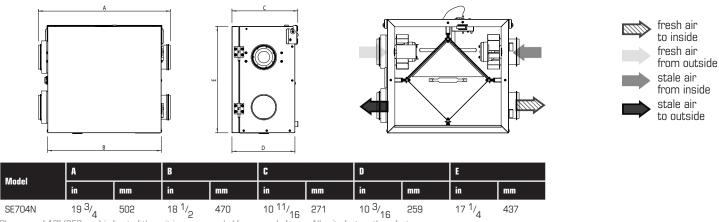
Clearance of 10" (250 mm) in front of the unit is recommended for removal of core. All units feature three foot plug-in power cord with 3-prong plug.
