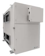
The SHR 1400 Commercial Heat Recovery Ventilation system (HRV) complements today's tight buildings. Fantech Heat Recovery Ventilators (HRV) are designed to supply air into a building while exhausting an equal amount of contaminated air to the outside. The aluminum heat exchanger core transfers sensible energy between air streams resulting in tempering of the supply air and reduced loads on the HVAC system.
