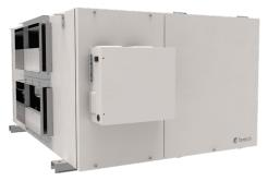
The SHR 1200 Commercial Heat Recovery Ventilation system (HRV) complements today's tight buildings. Fantech Heat Recovery Ventilators (HRV) are designed to supply air into a building while exhausting an equal amount of contaminated air to the outside. The aluminum heat exchanger core transfers sensible energy between air streams resulting in tempering of the supply air and reduced loads on the HVAC system.
