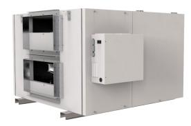
The SHR 700 Commercial Heat Recovery Ventilation system (HRV) complements today's tight buildings. Fantech Heat Recovery Ventilators (HRV) are designed to supply air into a building while exhausting an equal amount of contaminated air to the outside. The aluminum heat exchanger core transfers sensible energy between air streams resulting in tempering of the supply air and reduced loads on the HVAC system.
