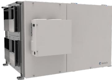
The SHR 450 Commercial Heat Recovery Ventilation system (HRV) complements today's tight buildings. Fantech Heat Recovery Ventilators (HRV) are designed to supply air into a building while exhausting an equal amount of contaminated air to the outside. The aluminum heat exchanger core transfers sensible energy between air streams resulting in tempering of the supply air and reduced loads on the HVAC system.
