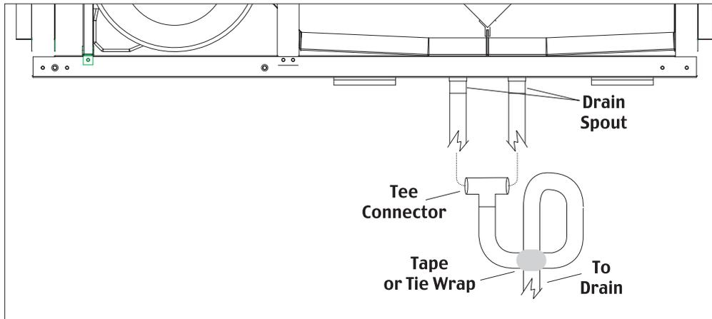
**!** If outdoor air temperature is above 32°F (0°C) at the extract air (30% RH/72°F, 30% RH /22°C), no drain line installation is required. If this is the case keep the drain spout as shipped from factory with the cap.
