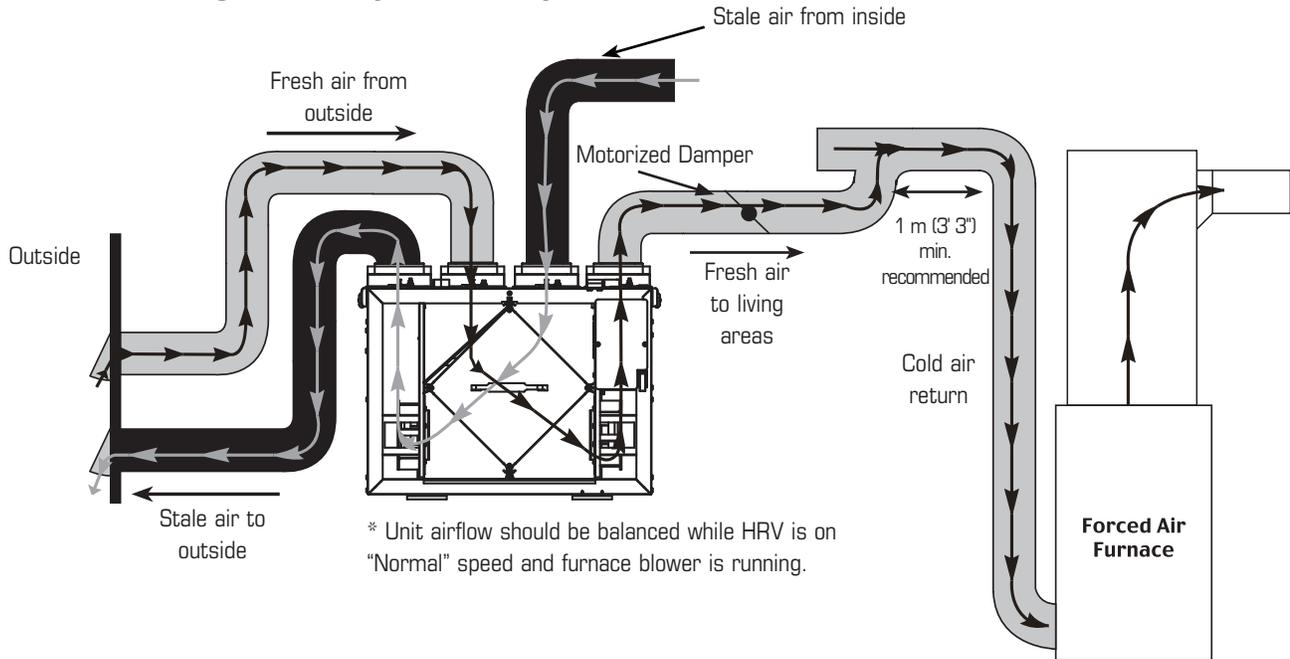
\* Unit airflow should be balanced while HRV is on "Normal" speed and furnace blower is running.
