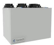
Fantech's VER 100 is an Energy Recovery Ventilator designed for higher static pressure applications. The unit brings a continuous supply of fresh air into a home while exhausting an equal amount of contaminated air. The energy recovery core at the center of the unit transfers heat and moisture from incoming air to the outgoing air that was cooled and dried by the building's air conditioner.
