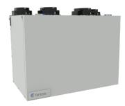
Fantech's, VER 200 is an Energy Recovery Ventilator designed for higher static pressure applications. The unit brings a continuous supply of fresh air into a home while exhausting an equal amount of contaminated air. The energy recovery core at the center of the unit transfers heat and moisture from incoming air to the outgoing air that was cooled and dried by the building's air conditioner.
