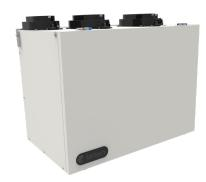
Fantech's, VER 200 is an Energy Recovery Ventilator designed for higher static pressure applications. The unit brings a continuous supply of fresh air into a home while exhausting an equal amount of contaminated air. The energy recovery core at the center of the unit transfers heat and moisture from incoming air to the outgoing air that was cooled and dried by the building's air conditioner.
