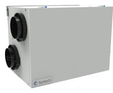
Fantech's, SER 150 is an Energy Recovery Ventilator designed for higher static pressure applications. The unit brings a continuous supply of fresh air into a home while exhausting an equal amount of contaminated air. The energy recovery core at the center of the unit transfers heat and moisture from incoming air to the outgoing air that was cooled and dried by the building's air conditioner.
