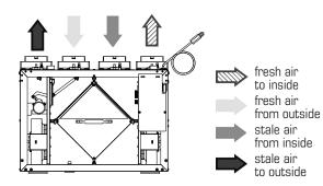
437 Clearance of 17" (432 mm) in front of the unit is recommended for removal of core. All units feature three foot plug-in power cord with 3-prong plug.
