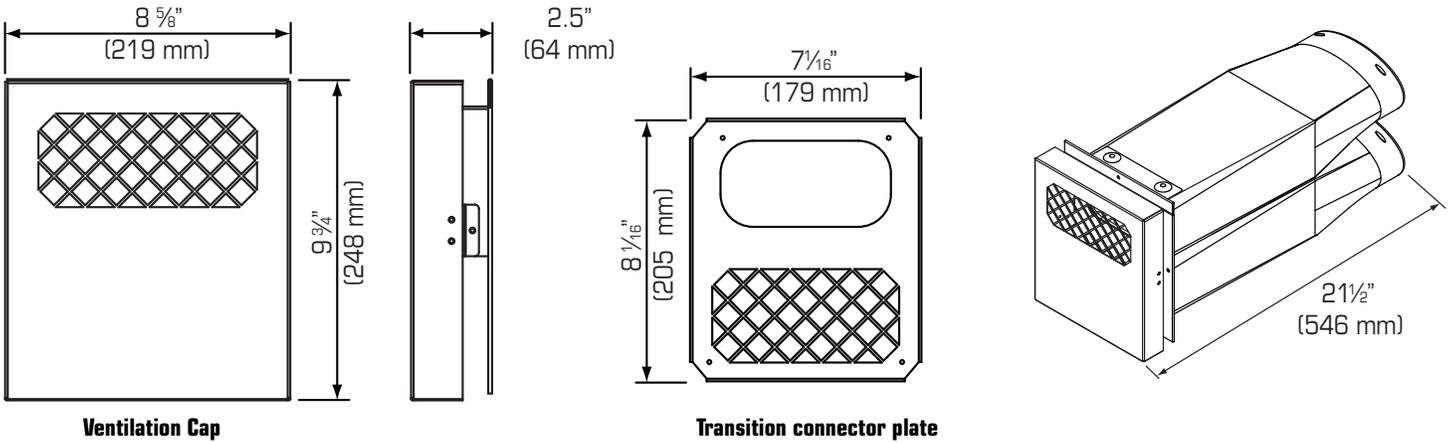
**Clearance – Assembled Transition Ducts**
