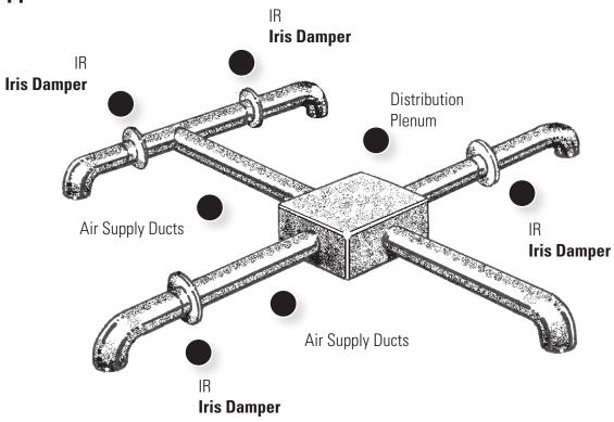
Typical multi-duct installation where Iris Dampers are used to balance the system.
