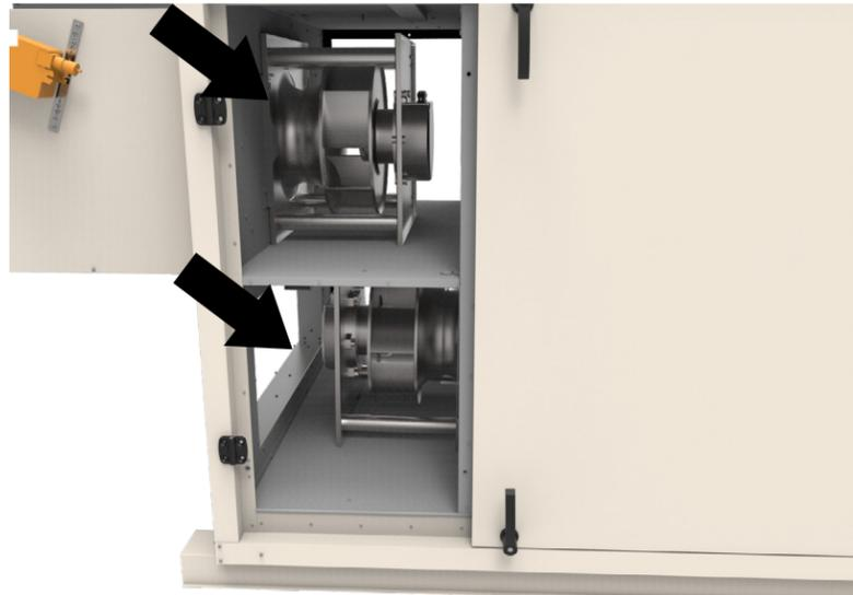
The speed of these EC fan motors are controlled by analog outputs from the unit controller. With feedback from the unit's built in pressure transducer modules, the controller will modulate the fan speed in order to maintain the airflow set point. This method of controlling the unit airflow is called Constant Air Volume (CAV). More details in the "Pressure transducer modules" section.
