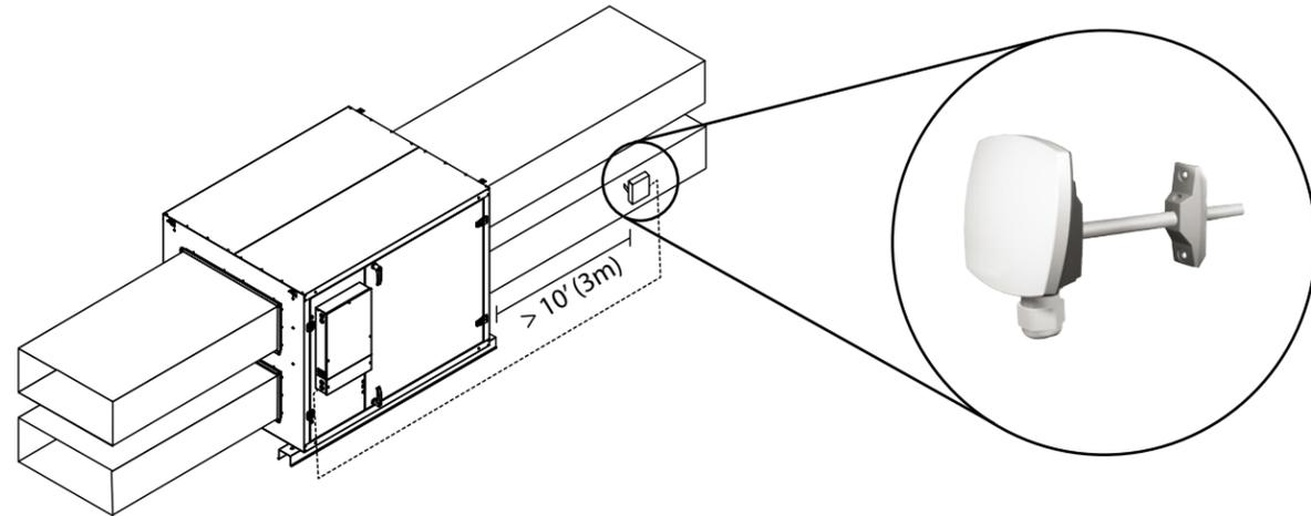
**!** The supply air sensor must be installed and wired back to the electrical connection box as indicated above for the unit to function. Ensure this is done before proceeding.
