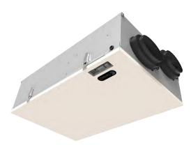
With a profile of only 8.75" high, Fantech's FIT 120E is ideally suited for condos and apartments that have no mechanical room and where it must be located over a false ceiling. The FIT 120E brings a continuous supply of fresh air into a home while exhausting an equal amount of contaminated air. The energy recovery core at the center of the unit transfers heat and moisture from the incoming air to the outgoing air that was cooled and dried by the building's air conditioner.
