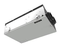
With a profile of only 8.75" high, Fantech's FIT 120E is ideally suited for condos and apartments that have no mechanical room and where it must be located over a false ceiling. The FIT 120E brings a continuous supply of fresh air into a home while exhausting an equal amount of contaminated air. The energy recovery core at the center of the unit transfers heat and moisture from the incoming air to the outgoing air that was cooled and dried by the building's air conditioner.
