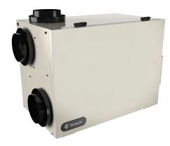
The SHR 3005R's double core configuration provides the greater thermal efficiency needed for homes being built to a higher energy standard. The incoming air passes through a first, then a second heat exchanger to provide maximum heat recovery. During winter, fresh incoming air is tempered by the heat that is transferred from the outgoing air so you save on energy costs, while during summer, the incoming air is precooled if the house is equipped with an air cooling system.
