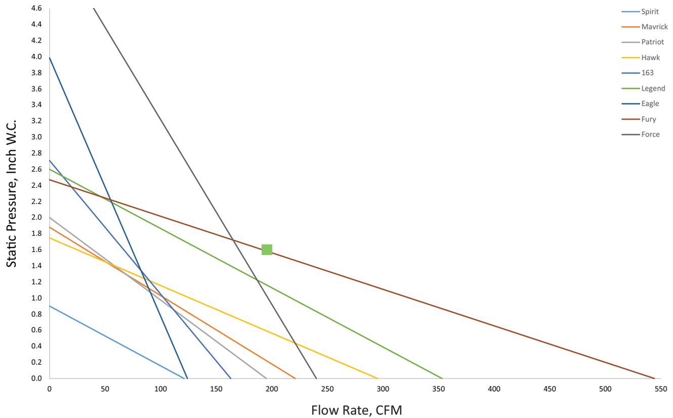
f. Overlay fan manufacturer performance curves (provided) over Working Point Graph and select a fan that performs equal or better than your system Working Point; Rn4 in this example.
