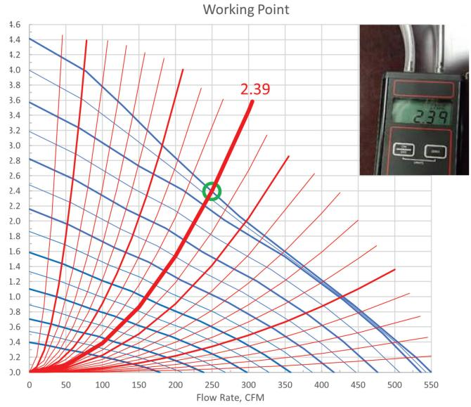
b. Plot fan performance curve for RPM ratio; thick blue curve
